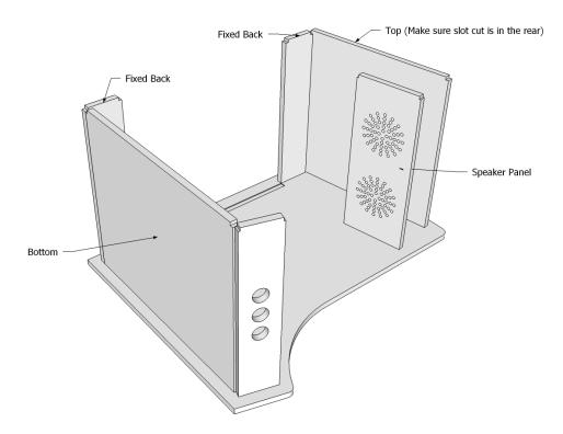
Step 5: Place the other side on top, but **do not glue**! Guide the tabs into the slots on the slide you place on top. Once complete, place a weight on top. Use a wet rag or paper towel and wipe up any excess glue that comes out of the slots. Let dry (overnight preferred).
