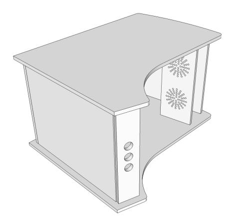
Step 6: After glue has dried, remove weight, take the left side off and place it down with the pockets up. Place glue in the pockets marked red in step 2. Carefully turn the right side assembly (right side and panels) over and guide the tabs into the correct slots. Once panels and slots are aligned, place a weight on top again, and wipe up the excess glue. You can now glue the batons into the 4 remaining shallow slots (2 on each side) and let everything dry (overnight preferred).
