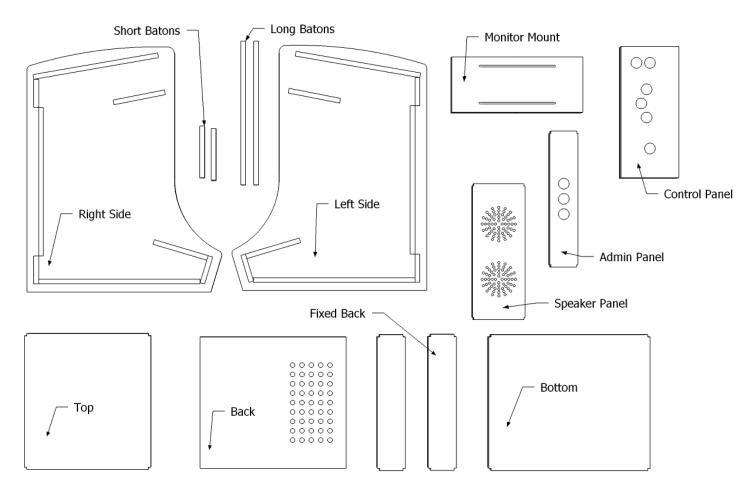
Step 2: Lay the right side down on your dropcloth, pockets up, and put wood glue into the slots that are colored **red only**. Fill each slot just under half full with glue. Excess will be wiped up later.
