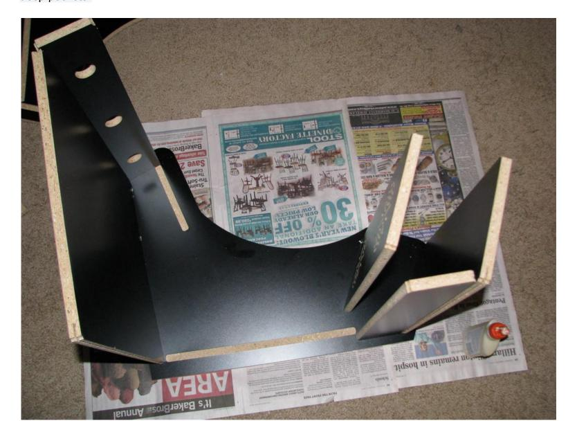
Place the other side on top (with NO glue yet), aligning the tabs into the slots:
