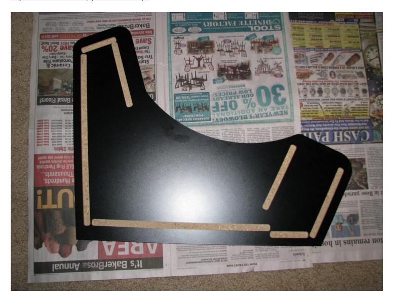
Fill each of the five 1/4" deep pockets with a **liberal** amount of wood glue. Don't be stingy. Insert each of the tabbed panels into the deep pockets:
