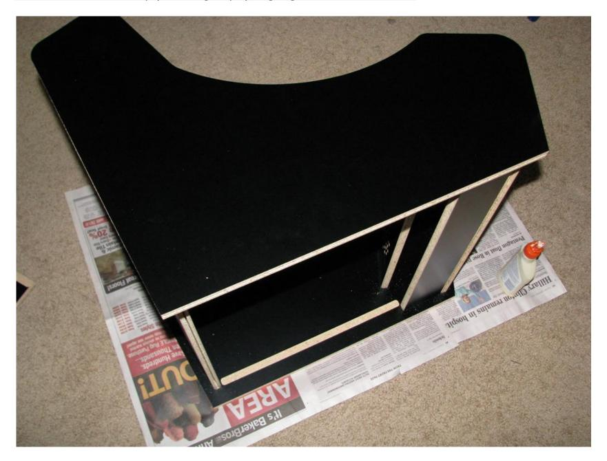
Place a heavy weight on top, wipe up the excess glue with a damp paper towel. Wait for an hour or so.
