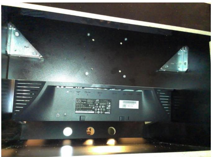
Usually the monitor is enough to hold the bezel plexiglass in place.
