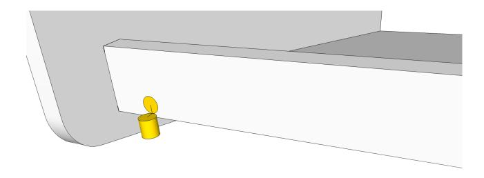
Close both hinges so they stick straight out from the panel. At this time, take the control panel assembly, line up the holes on the admin panel with the barrel hinges, and press the control panel onto the hinges.
