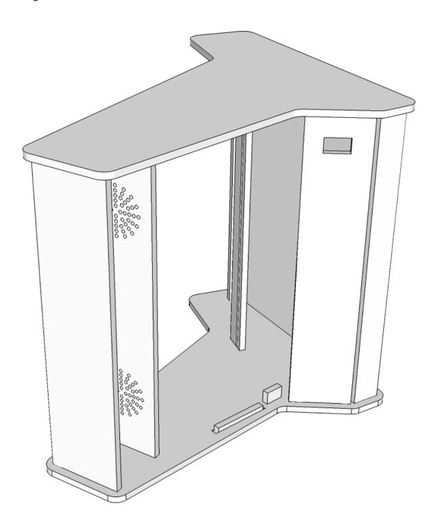
Once the glue has dried overnight, remove the weight and remove the side that wasn't glued. Place that side down on a flat surface, slots facing up, and add glue into the slots. Carefully turn over the glued side / panels assembly and insert the tabs into the correct slots, press down, add a weight, and wipe up any excess glue. Also insert the remaining Baton and Back Door Latch Mount. Let dry overnight.
