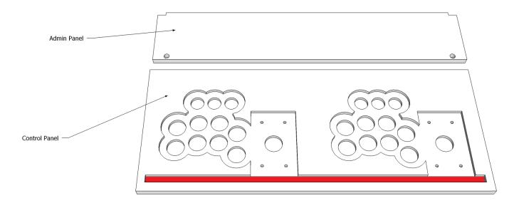
Insert tab of the Admin Panel in to the slot on the Control Panel as shown. Make sure the small holes at the bottom of the Admin Panel are facing the back of the Control Panel! Press down to ensure correct fit. Wipe up and excess glue and let dry overnight.
