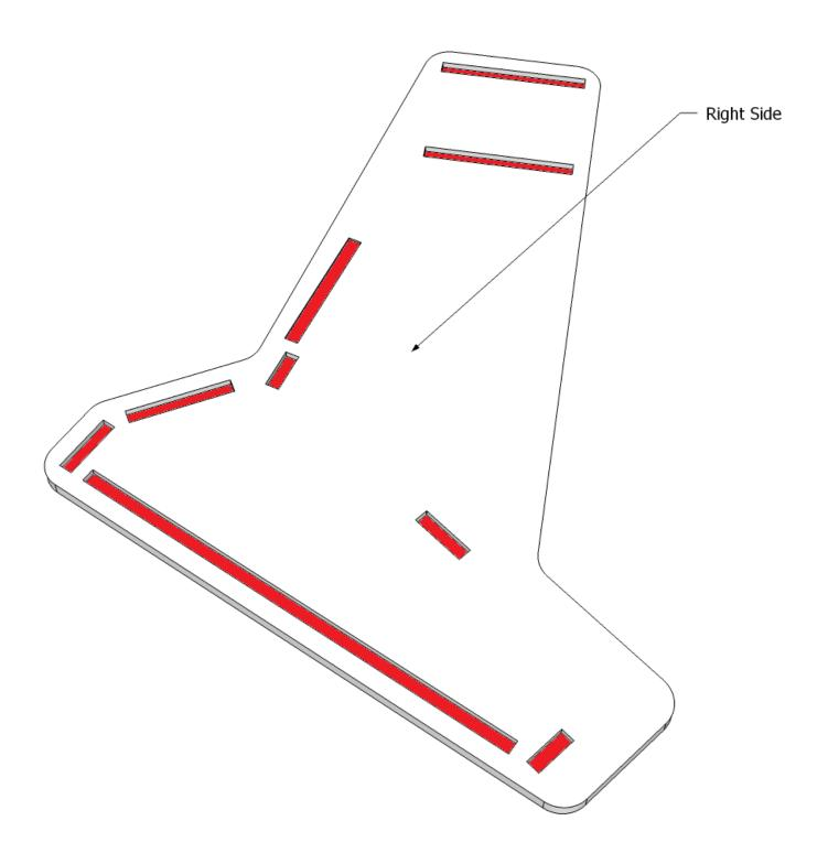
Insert the Control Panel Assembly Hinge Panel into the Right Side as shown. Make sure that two small holes are near the bottom and facing out:
