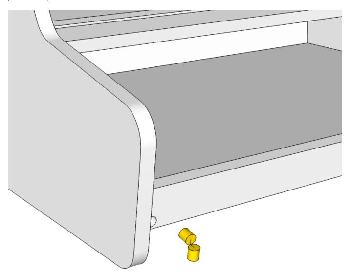
Insert the barrel hinge into the hole on the cabinet. Ensure that the open part of the hinge still faces down. Repeat for both sides of the cabinet.
