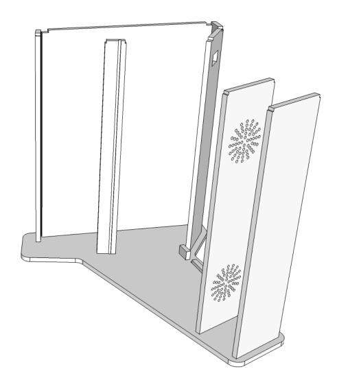
Carefully place the remaining side on top (no glue at this time) and line up all the tabs into the slots. When the tabs and slots are aligned, press down. Place a weight on top of the side to apply pressure. Take this time to wipe up any excess glue that may seep from the slots. Let dry overnight.
