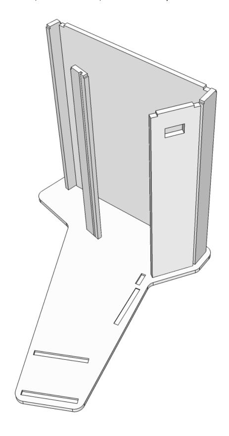
Insert Baton and Back Door Latch Mount into the side as shown.
