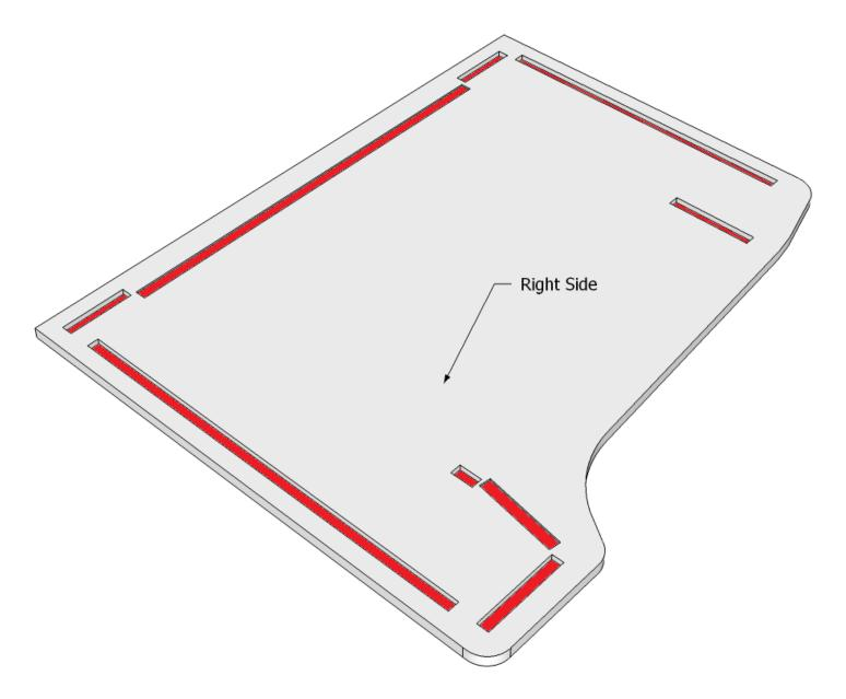
Insert the Admin Panel and Bottom Panel into the Right Side. Make sure that speaker cutout is near the top:
