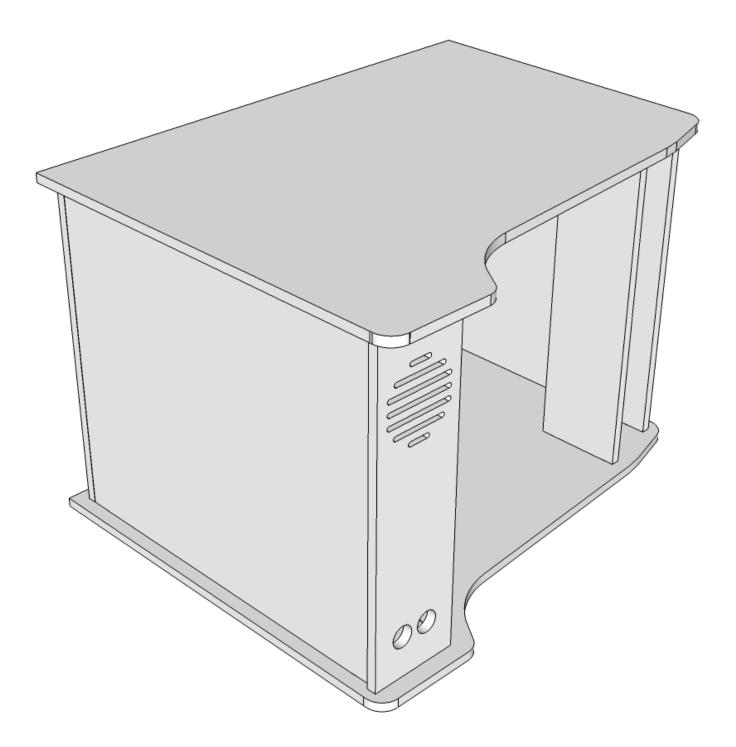
Once the glue has dried overnight, remove the weight and remove the side that wasn't glued. Place that side down on a flat surface, slots facing up, and add glue into the slots. Carefully turn over the glued side / panels assembly and insert the tabs into the correct slots, press down, add a weight, and wipe up any excess glue. Also insert the remaining batons. Let dry overnight.
