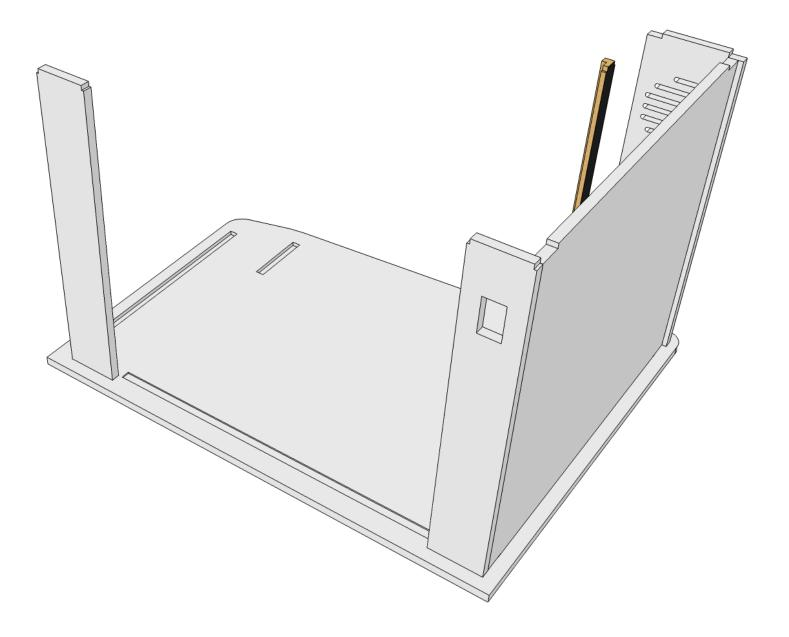
Install the Top Panel and the Lower Marquee Panel as shown. Make sure the T-molding slot cut in the Top Panel faces the rear of the cabinet.
