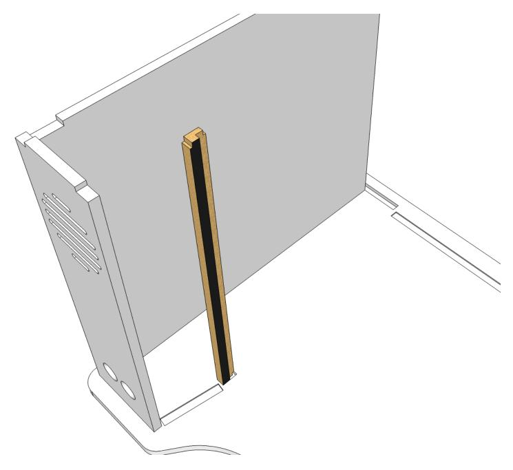
Insert the Upper Back and Lower Back Panel as shown:
