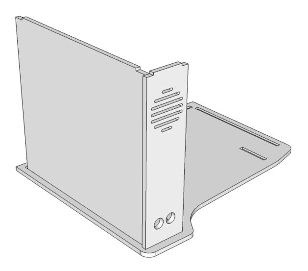
Next, insert the Bezel Shelf Panel as shown, with the plexi slot facing UP and closest to the rear of the cabinet (note the part has been colored to help with visualization):
